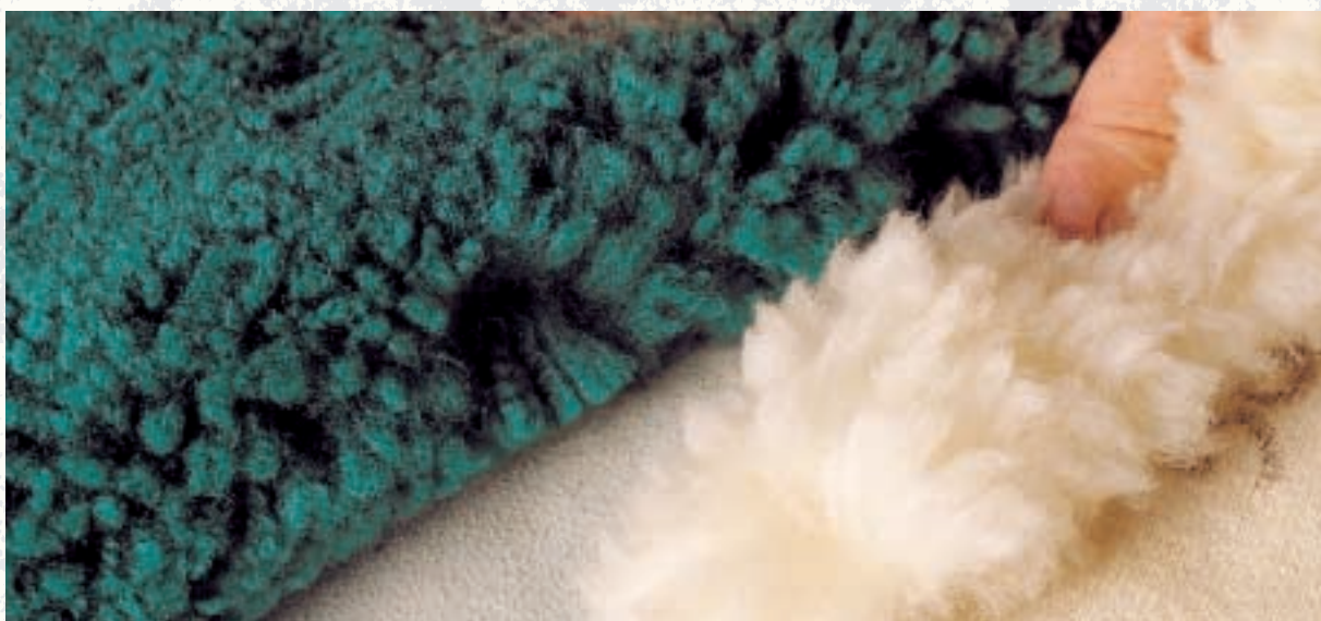
The pile of an Australian Medical Sheepskin, compared to an imitation product (often a polyester pile knitted onto a synthetic fabric).
