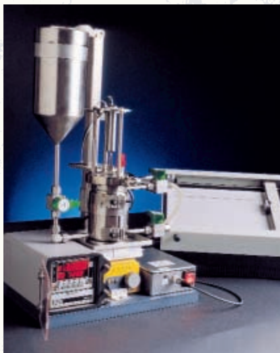
CSIRO developed machine for testing the stability of leather at high temperatures.
